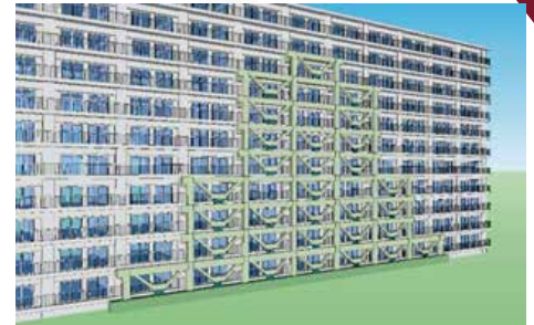
Image of SUMAIRU Damper Frame reinforcement
