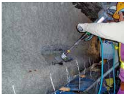
Concrete core extraction by drilling
